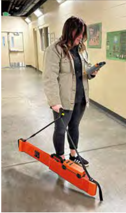
Historic Preservation Specialist Erica Scherr demonstrates the agency's new electromagnetic induction meter.
